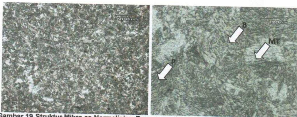
Gambar 19. Struktur Mikro as Normalising-Pemanasan I 650 - Pemanasan II 650
